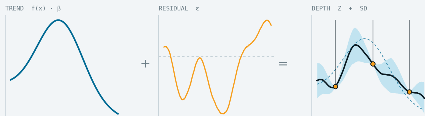
Fig. 03 · Schematic. Prediction uncertainty collapses at the wells and grows away from them, at a rate set by the variogram.
